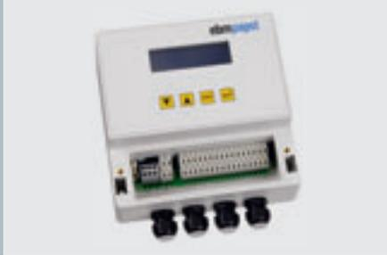
Stand-alone control device for refrigeration and air-conditioning technology in conjunction with the corresponding sensors. Using the controlled 0–10 V output or RS485 MODBUS RTU connection, ebm-papst fans with a corresponding input can be triggered. The function includes multifunctional pressure and temperature control as well as display and entry of various parameters. The integrated LCD display provides easy operation across multiple levels.
